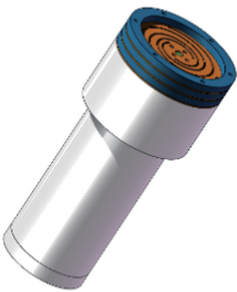
Fig. 31 3D model of vibration isolator
